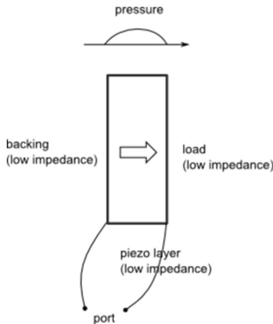
Low impedance at both side of plate indicate resonance at plate thickness  $n\lambda/2$ .
