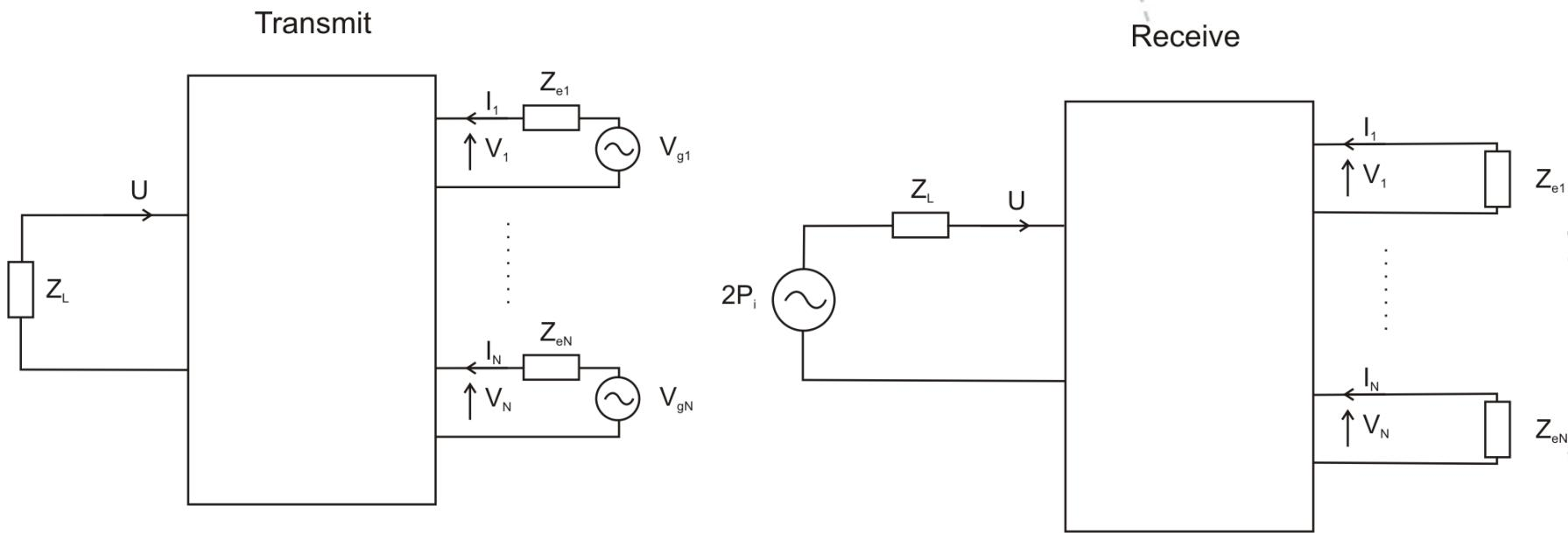
$$\begin{bmatrix} I_1 \\ \vdots \\ I_N \\ U \end{bmatrix} = \begin{bmatrix} Y_{11} & \cdots & Y_{1N} & H_{tt,s,1} \\ \ddots & \ddots & \vdots & \vdots \\ Y_{N1} & \cdots & Y_{NN} & H_{tt,s,N} \\ H_{tt,s,1} & \cdots & H_{tt,s,N} & Y_m \end{bmatrix} \begin{bmatrix} V_1 \\ \vdots \\ V_N \\ 2P_i \end{bmatrix}$$
